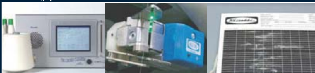
Yarn clearing system
